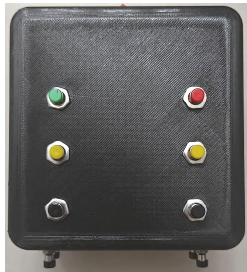
Figure 4 Six-button Braille input interface in standard two-column, three-row cell layout
